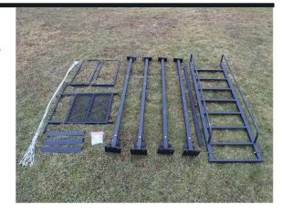
You will need the following tools to assemble your stand.... Level, band cutter to cut the strapping holding the kit together, 3/4 wrench, ratchet or impact gun with 1/2 inch socket, ratchet or impact gun with 3/4 inch socket.
